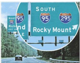
Traffic sign viewed from a 12 degree field of view with 3x keplerian bioptic
